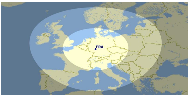
Figure 3.3: Operational range of hydrogen aircraft based at Frankfurt, refuelling at home base only (ranges of 400 Nm and 800 Nm) (Source: www.gcmap.com )
